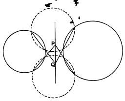
Draw any circle cutting the given circles in real points, and let the radical axes, that is the common chords, of these circles intersect in the point P. Then P is a point on the radical axis of the given circles.
